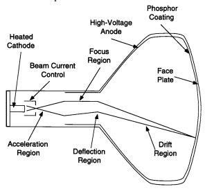
Figure 1 - Cathode Ray Tube (CRT)
